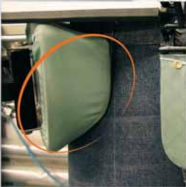
device for the simultaneous steaming press of flap and front pockets for three pressing operations in just one cycle
