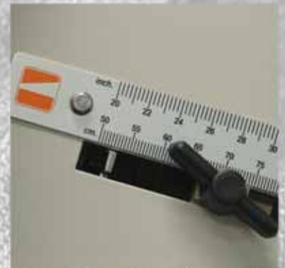
adjustment of the trouser top and legs sizes with mechanic stop for stretch-fabrics and automatic signal of out of size
