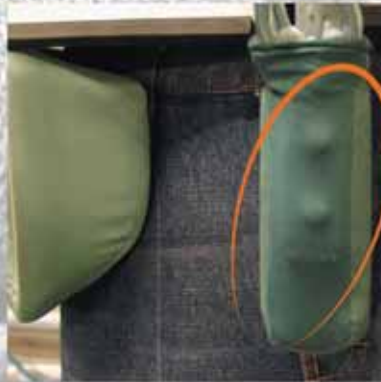
device for the simultaneous steaming press of flap and front pockets for three pressing operations in just one cycle
