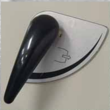
manual control placed in the side of the machine for vacuum adjustment
